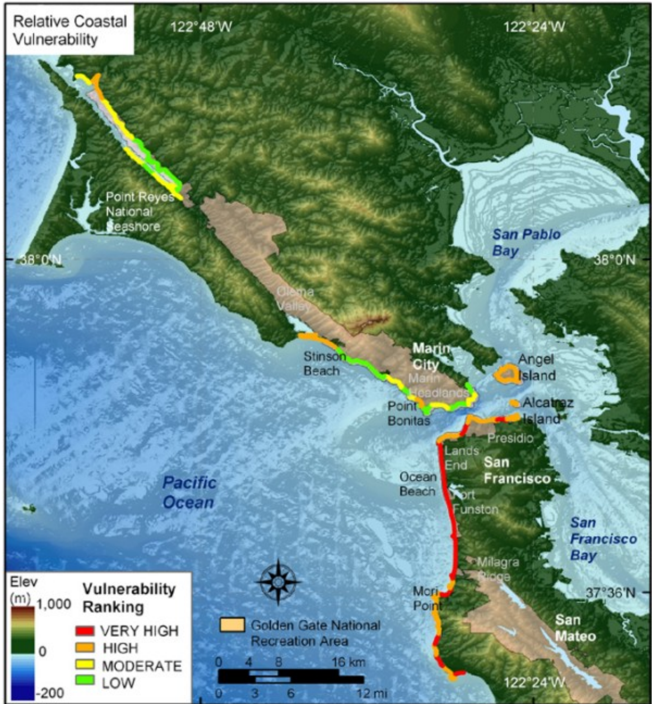
Figure 19. Relative coastal vulnerability for Golden Gate National Recreation Area. The colored shoreline is the relative coastal vulnerability index determined from the six variables. The “very high” vulnerability shoreline is found along sandy beaches where wave heights are highest and coastal slope is low. The “low” vulnerability shoreline is found along rocky cliffs where wave heights are lower and coastal slope is steep (Pendleton et al. 2005a).
